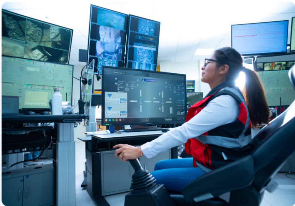
The Integrated Operations Centre (IOC) at Quellaveco is a remote command and control hub that uses real-time data to manage and optimise the mine's operations. It allows for the remote control of autonomous mining trucks and drills, improving safety by moving operators away from hazards. Pictured: Carla Rubio Pacco, co-ordinator in the IOC at Quellaveco.
