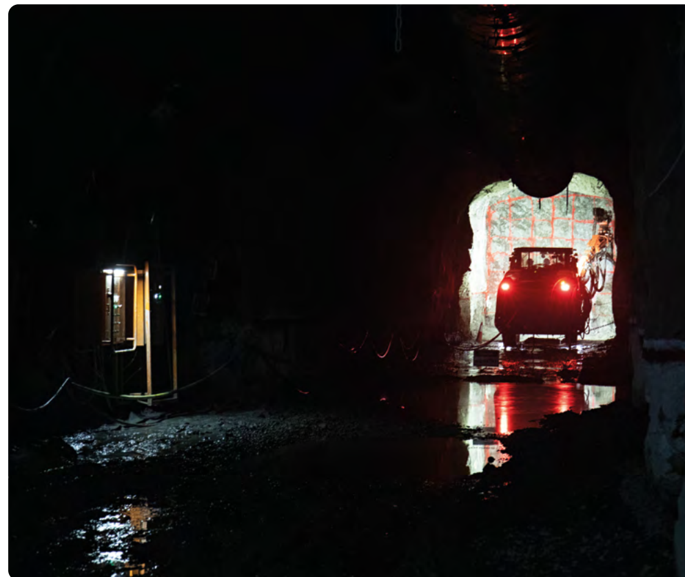
Venetia, South Africa's premier diamond mine, is transitioning from open pit to underground mining. Clearly visible in front of the drill rig is the high-tensile steel mesh that is applied, ahead of drilling, on stope roofs and walls to protect operators in the development area.
